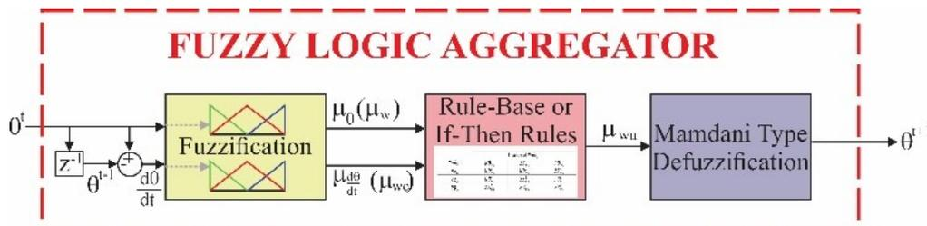
**Figure 1.** Proposed aggregation method similar to fuzzy logic controller.
